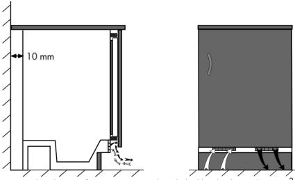
To avoid any loss in performance, air suction channels should not be obstructed. (140 cm<sup>2</sup>)
